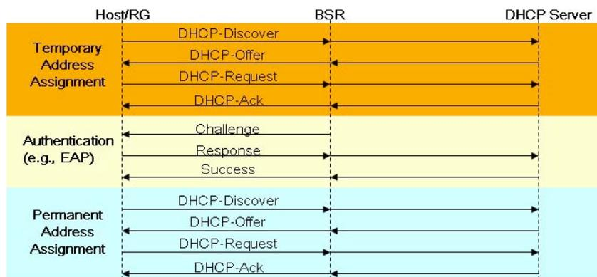
Figure 11: IPoE Authentication Using Temporary IP Address Assignment
